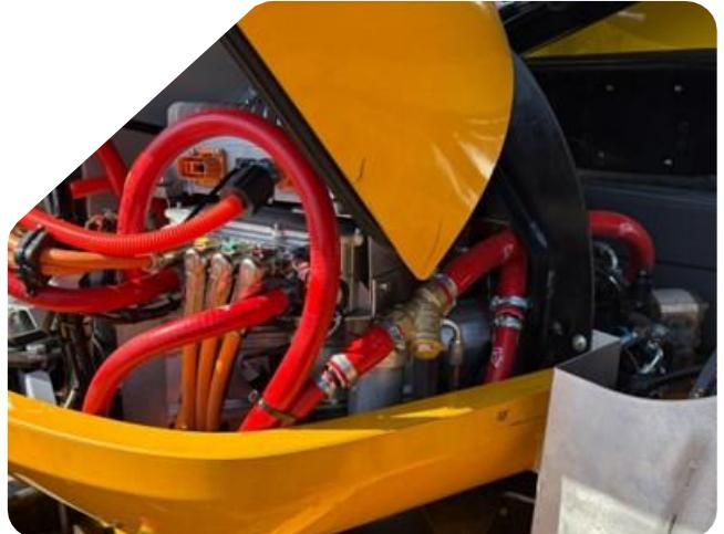
The motor is shown integrated with both a new off-the-shelf hydraulic gear pump using standard fittings, and an existing vehicle pump—demonstrating its flexibility for new designs as well as retrofit applications. This adaptability enables seamless integration across a range of platforms and use cases.
